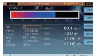
DVB-S/S2 Signal Measurement
