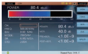
QAM signal quality measurement
