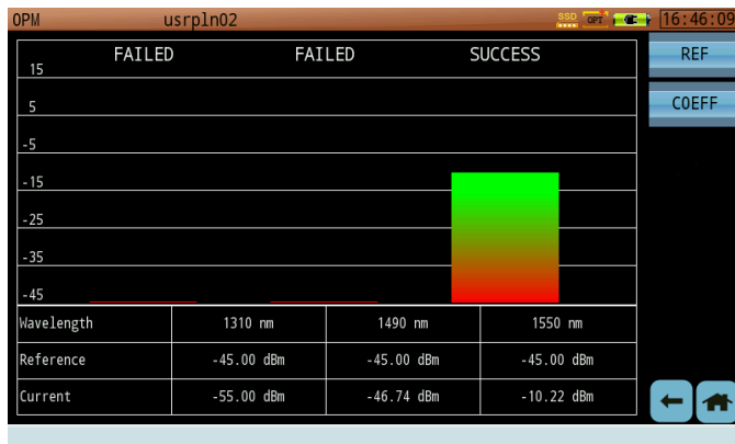
Figure 20: Optical Power Measurement
