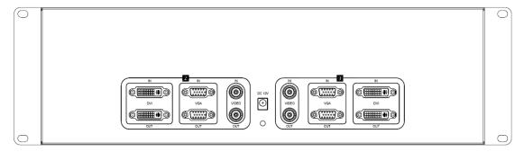
**Note:** The interfaces included in Monitor 1 are the signal interface for Monitor 1. The interfaces included in Monitor 2 are the signal interface for Monitor 2. The power interface is common / public interface for both Monitor 1 and Monitor 2.
