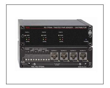
**APPLICATION:** The RU-TPS4A is a four output audio sender, signal and power distributor module compatible with RDL Format-A twisted pair products. Three line-level sources may be connected to the module using the +4 dBu balanced detachable terminal block. Studio-quality buffer amplifiers feed the three pairs of the four rear-panel RJ45 **OUTPUT** jacks at the correct operating level.
