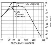
BOOST ADJUST Adjust for desired low frequency boost. This control is factory set to match the JBL Model 4645 THX approved subwoofer (THX is the registered trademark of Lucasfilm, Ltd.). This is a 25-turn control which sets the boost at 30 Hz. It may be turned counterclockwise for subwoofers not requiring this boost.
