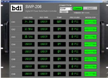
BDI's free graphical user interface is a compact resident program that allows the user to configure the name of each channel and provides status of each channel forward/reflected power, temperature and line pressure.
